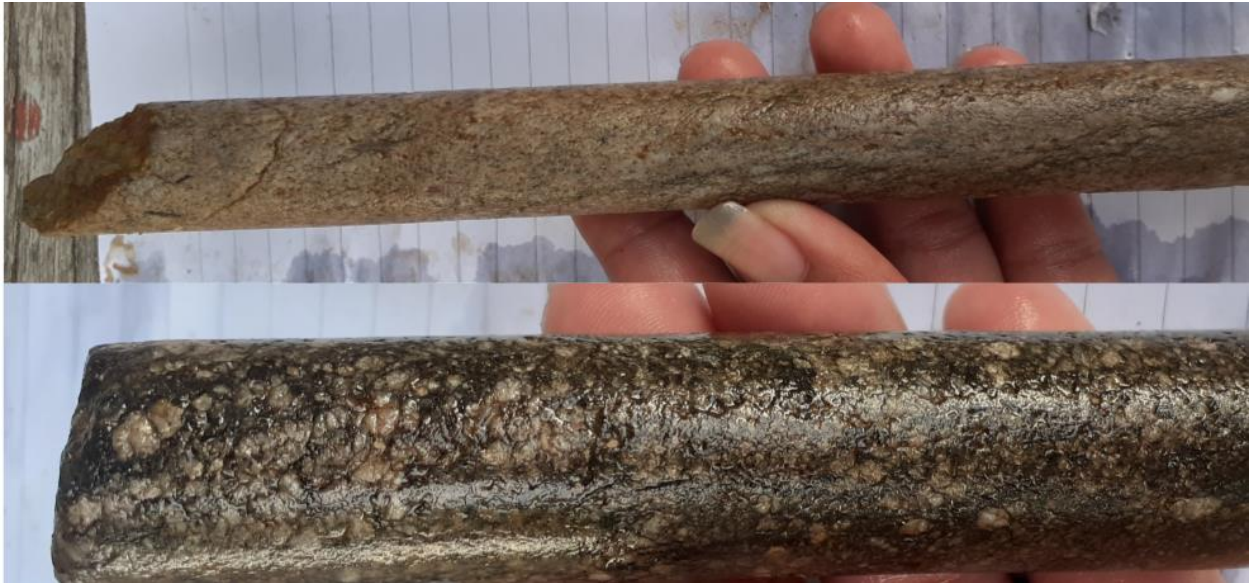
Figure 10. Some typical drill cores of metasedimentary rocks (LA91 no. 129-130-132, depth 27-30m)
