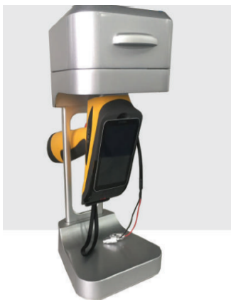
Figure 2 A benchtop pXRF (Skyray Instruments, n.d.)
