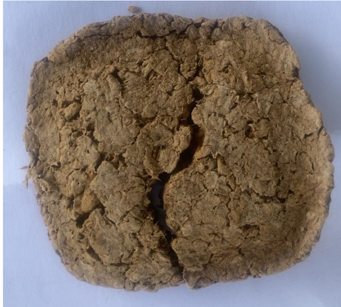
Figure A 1: Control Sample after adding water: 100% waste cardboard
