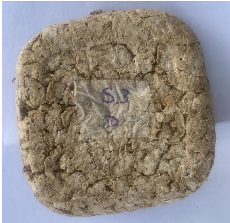
Figure A 4: Sample after adding to water: modified 85%:15% cardboard: Starch
