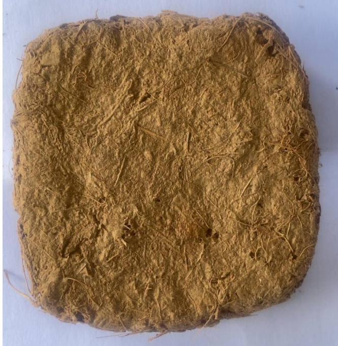
Figure A 9: Sample after adding to water: modified 50%:50% cardboard: coconut fibers
