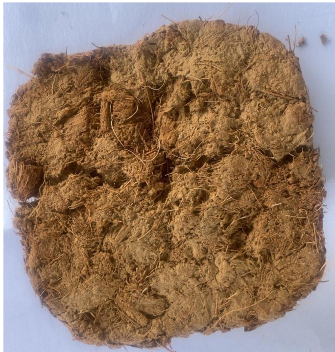
Figure A 2: Sample after adding to water: unmodified 90%:10% cardboard: coconut fibers
