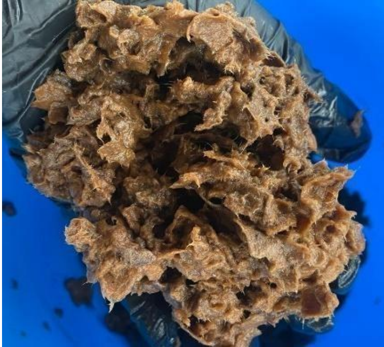
Figure 9: Blended waste cardboard after soaking for 24 hours in tap water
