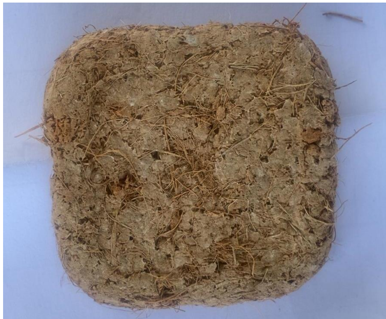
Figure A 6: Sample after adding to water: modified 75%:15%:10% cardboard: starch: coconut fibers
