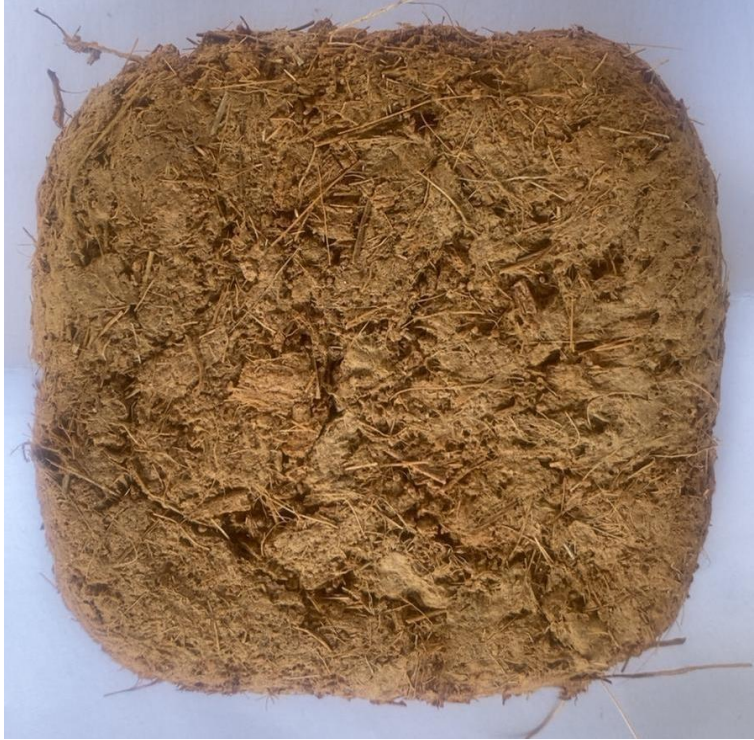
Figure A 7: Sample after adding to water: Modified 70%: 20%: 10%, Cardboard: Starch: Coconut fibers
