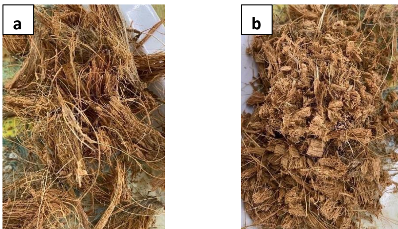
Figure 10: Coconut fibers directly segmented from the exocarp (a) and smaller chopped coconut fibers (b)
