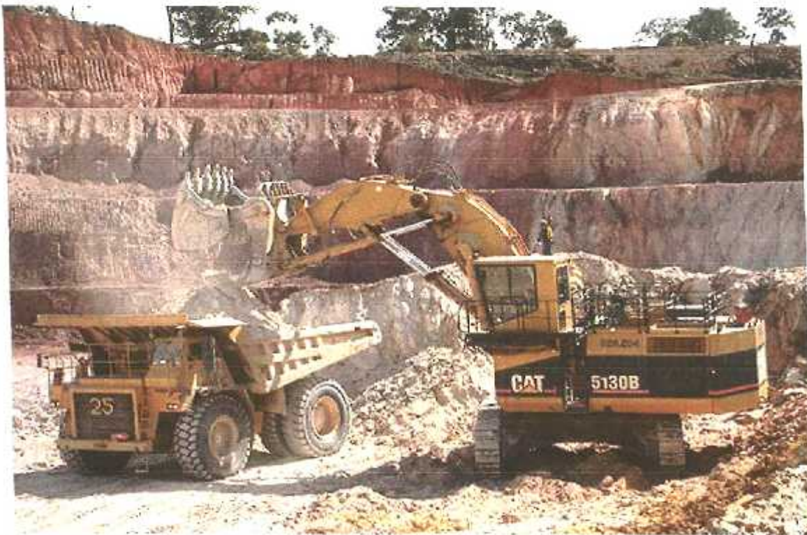
Figure 2.4: Hydraulic Shovel loading 777 haul truck at the mine site ( RGM)
