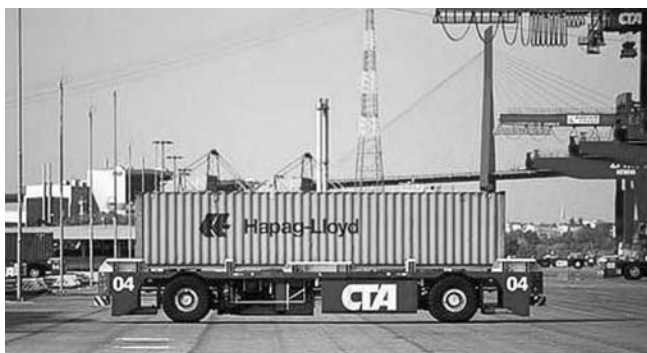
Fig. 1 AGV employed at the Container Terminal Altenwerder, Hamburg, Germany (source: http://www.hhla.de/de/Geschaeftsfelder/index.jsp , visited on August 22, 2005)
