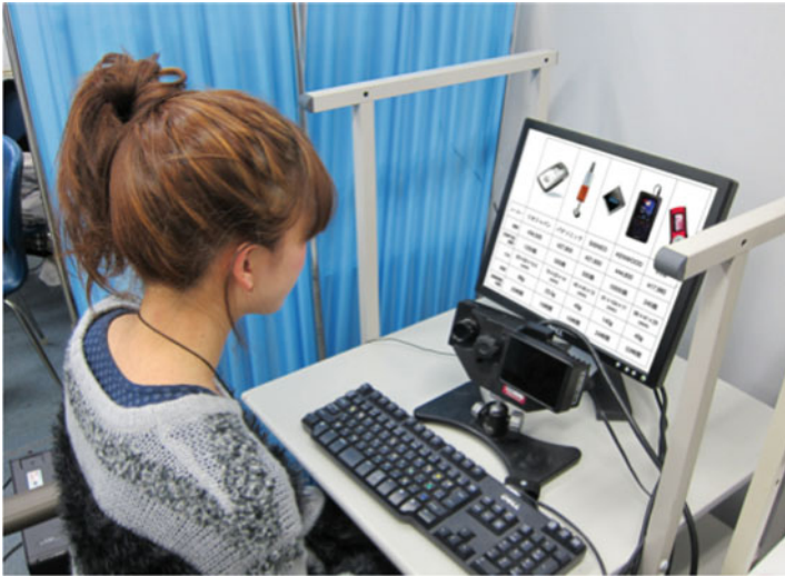
Fig. 13.4 Non-contact type of eye movement measurement system. Note: Eyelink 1000 Remote, product of SR Research. Source: Okubo and Takemura (2011)
