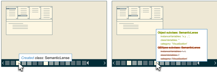
Fig. 5 Hovering shows which source code element has been changed (left). Holding shift in addition shows the full difference to the previous version (right)
