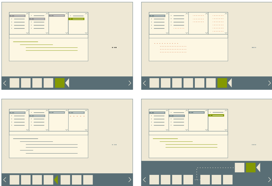
Fig. 4 (From top left to top right) A programmer modifies source code which implicitly creates items in the version bar. The programmer decides to withdraw several changes by going back to a previous version (bottom left), and continues working and creating new changes, which will appear on a new implicitly created branch (bottom right)
